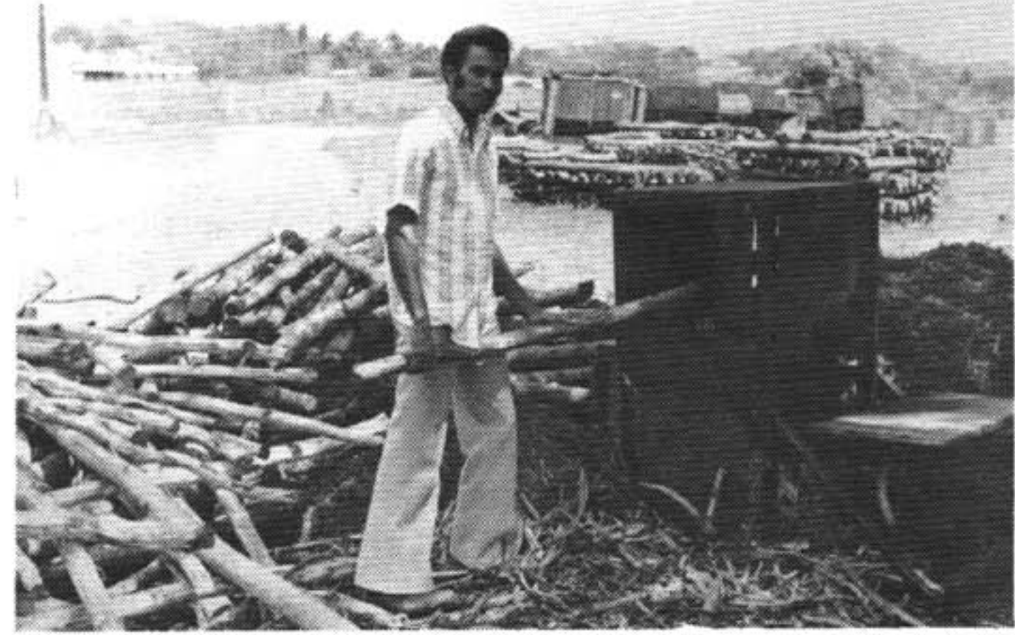
Removing the bark from Mahogany ( Swietenia spp.) posts prior to treating.
