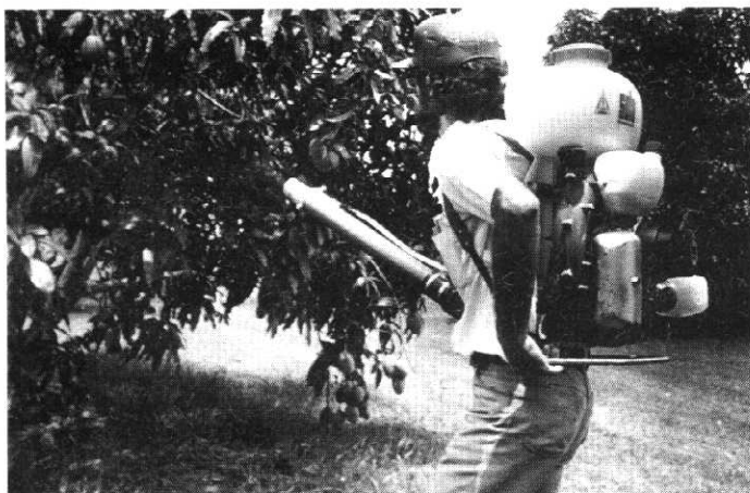
Making use of a back pack motorized mist blower can be a real help to farmers, as demonstrated at a field workshop.
