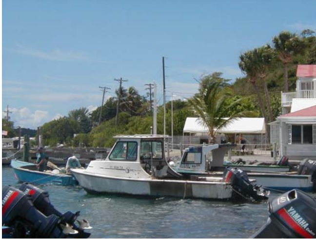
Photo 27: St. Thomas, USVI. Frenchtown commercial fishers' landing site. Boat in middle is a trap fishing boat with pot (trap) hauler. The metal sheet on side of boat is to protect the fiberglass when pots are hauled.
