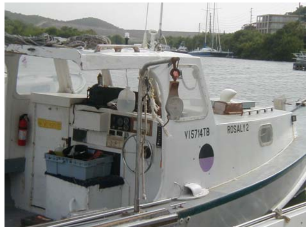
Photo 22: A typical pot hauler used to haul both fish and lobster traps.
