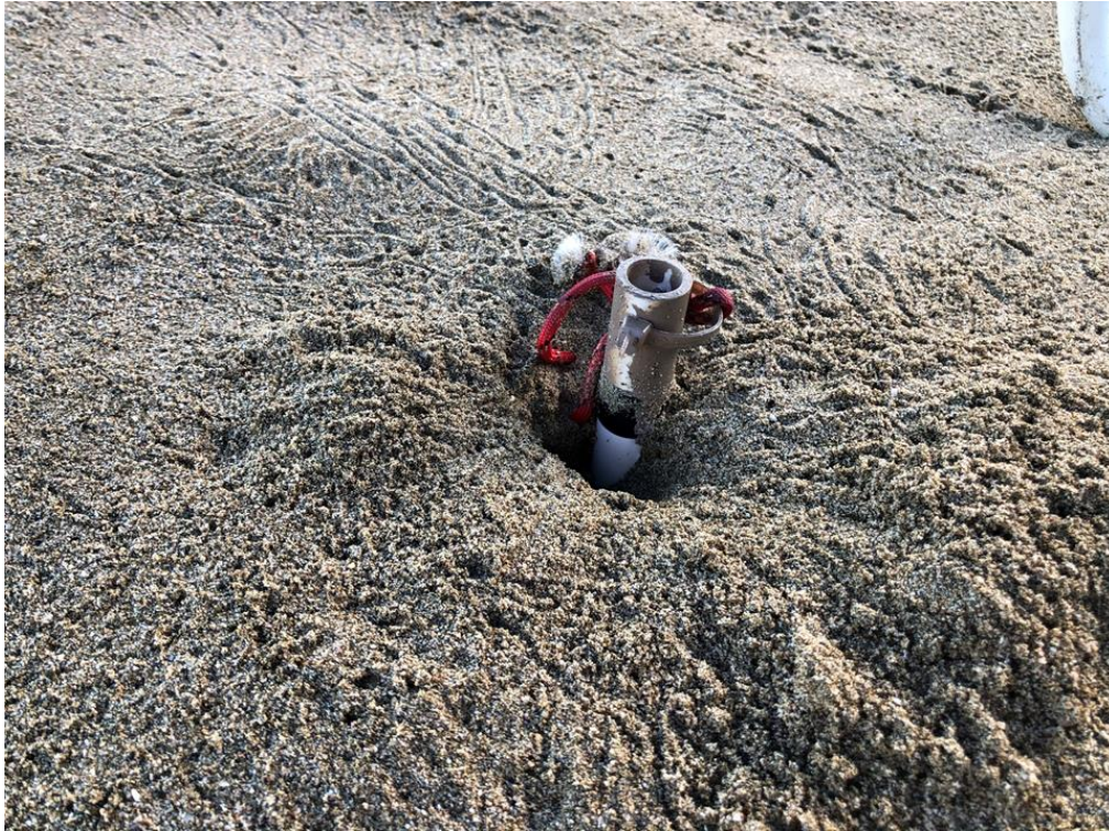
Figure 24: Ghost crab burrowing down a HOBOT logger installation. Photograph by Kaliegh Schlender.
